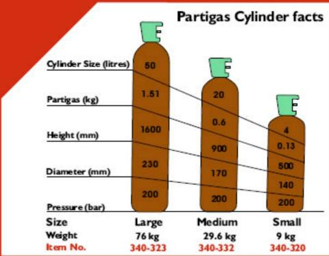
Using the diagrams, you can determine the most appropriate cylinder for your needs. Note that the diagrams show the approximate number of balloons that can be filled. Numbers will vary according to balloon manufacturer and the shape of the balloon.
